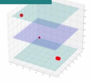
A 3D representation of the event is provided for an easier visualization of each event. Each plane denotes a detector plane. A red sphere is used to denote the places on the plane that a particle crossed. The size of these spheres are proportional to the energy this particles left on our detector.
