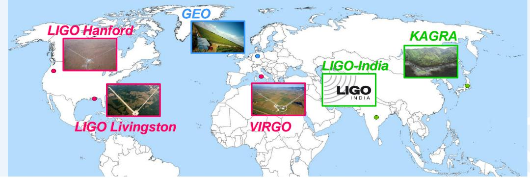
In order to locate the source of GWs and to better estimate its relevant parameters a network of gravitational wave detectors is needed
